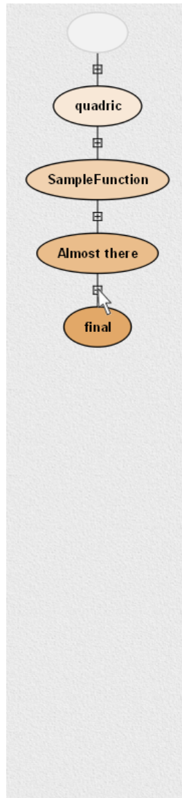
Figure 5.2: To conserve space, linear sequences of non-tagged nodes may be hidden from view.
